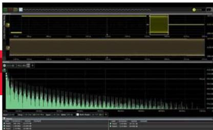
Fast Fourier Transform (FFT) includes powerful tools for extreme frequency domain (spectrum) analysis. Use the FFT to compute both magnitude and phase, and use multiple FFT windows, peak search and navigation, amplitude modulation, FFT mask triggers and gated FFT measurements to analyze waveforms.
