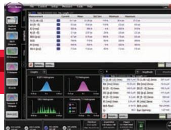
**Advanced jitter and amplitude analysis.** Accurate decomposition of impairments provides compliant total jitter (TJ) results and insight into root cause of eye closure.
