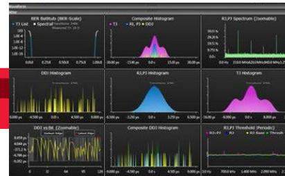
Get deep insight into your digital designs. EZJIT Plus features two methods to properly separate the jitter into random and deterministic components. If you have bounded uncorrelated jitter, simply use Keysight's new tail-fit algorithm; otherwise Keysight's spectral method and 75 fs of sample clock jitter ensure the most accurate measurement.
