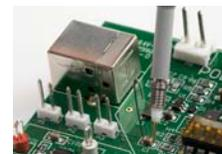
For example the N7020A power rail probe is an active probe designed specifically to measure DC voltage rails. With low noise, low loading, a large DC offset range and 2 GHz of bandwidth it enables you see the details of your signal without added noise of your measurement system.
