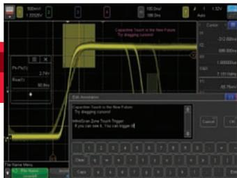
**Experience the capacitive 12-inch touch screen.** Drag measurements, cursors and sidebar panels for quick oscilloscope setup. Use the alpha-numeric touch pad for dramatically faster annotation.
