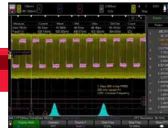
**Visualize signal integrity.** Features jitter analysis with clock recovery. Use serial and clock TIE measurements, and view jitter in various plots including jitter: histograms, trend, spectrum and statistics. Application also includes color-graded real-time eye analysis.
