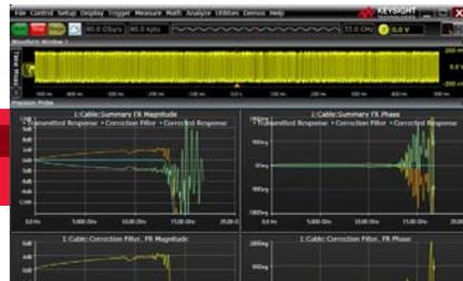
Use PrecisionProbe advanced to get full S21 characterization of cables up to 65 GHz, in addition to spectrum and complex modulation measurements. The simple network analysis saves you time and improves measurement accuracy by automatically compensating for both magnitude and phase loss caused by cables.
