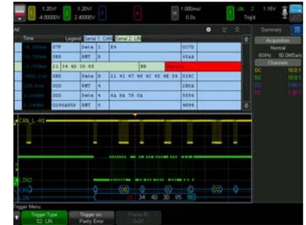
CAN/LIN triggering and hardware-accelerated decode helps you quickly find and debug errors and signal integrity problems on CAN and LIN serial buses.
