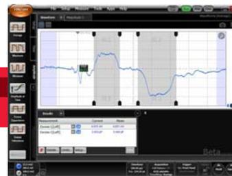
**Time domain reflectometer.** Measure both impedance and S-parameters, and verify transmission quality on cables, components and channels.
