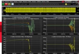
Quickly characterize and compensate the frequency response. PrecisionProbe uses its 200 GHz indium phosphide process to create a fast edge for characterization.
