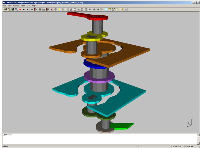
Figure 4: In a 3D view the designer can precisely visualize the transitions in and out of complex HDI vias
