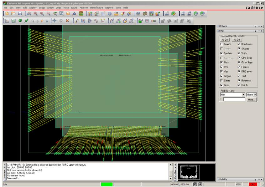
Figure 2: A multi-die stack on a BGA substrate viewed in 2D
