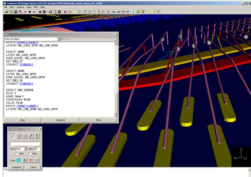
Figure 6: A design rule violation is highlighted using the info command. 3D visualization lets you see precisely where 3D spacing rules are violated
