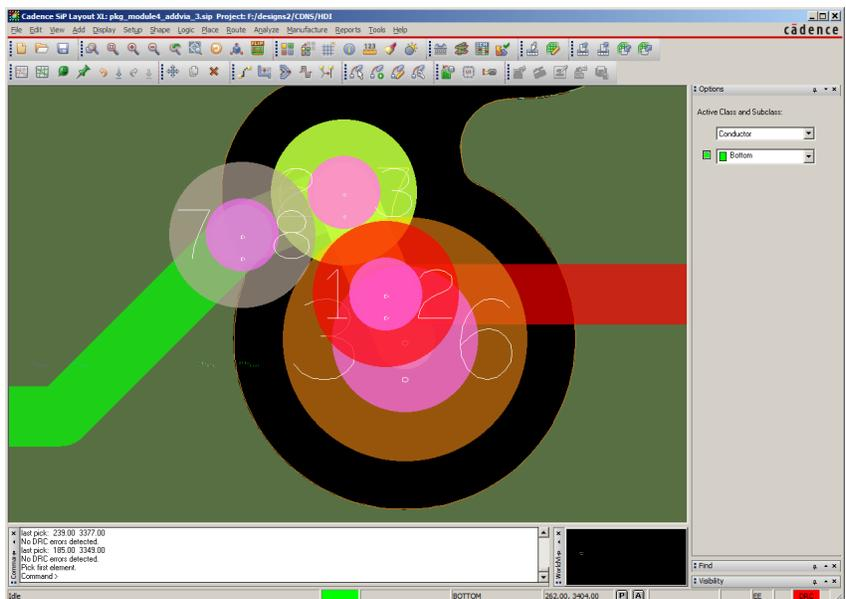
Figure 3: It is difficult to understand the connectivity path between the metal interconnect as it transitions between layers in 2D
