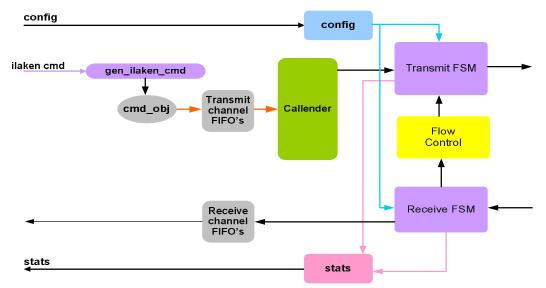
Receiver once it is in sync and deskew is done, then it collects all the frames/words and passed on to user. There are per channel fifo for user to collect the frames. There is
