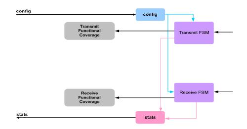
Monitor implements the functional coverage, which user can modify to add more coverage in object oriented way.
