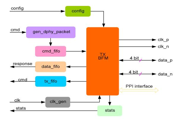
The transmitter can be made to abort in middle of transfer to check if receiver hangs, also transmitter can create various false start and bus idle conditions, insert ecc and checksum errors.
