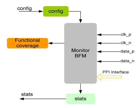
Monitor also keeps track of all the access on bus, and this stats can be accessed any time during simulation. Monitor implemented callbacks and functional coverage model.
