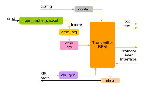
At each stage of the MPHY transmit FSM, callbacks are executed and user can use this callbacks to modify the behavior of the transmit FSM.
