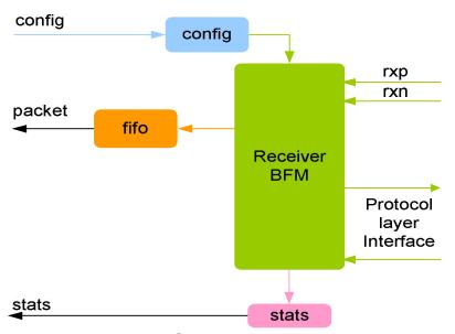
At each stage of the MPHY receive FSM, callbacks are executed and user can use this callbacks to modify the behavior of the receive FSM.
