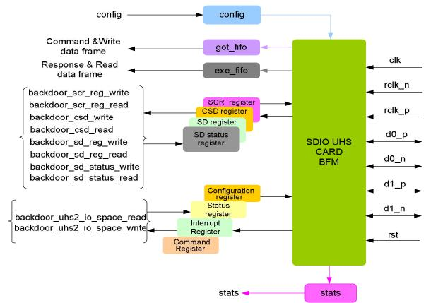
SDIO UHS-II card is first configured with different configuration parameters. The slave keeps monitoring the bus for a valid command from the host. Depending on command type slave responds to the HOST. For a write command, slave receives data from host and writes to internal memory model. For the read command, slave sends the data to host from the memory model or FIFO. Slave BFM behaves as per the device configured. At the end of command reception, status counters are updated.
